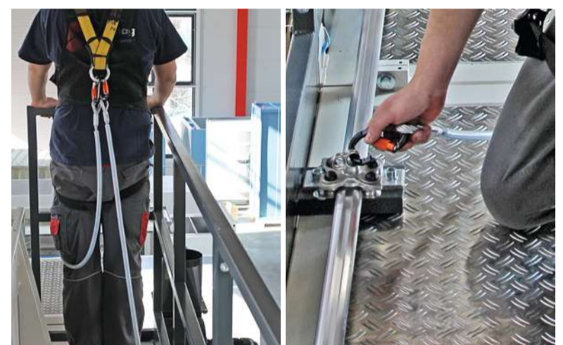
The hand rail on one side with mount fixing points brings increased safety
