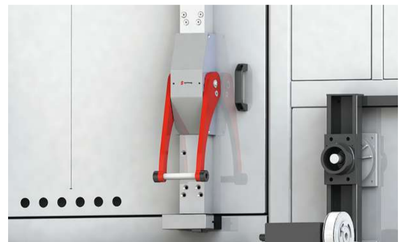
New locking mechanism on the drier doors
