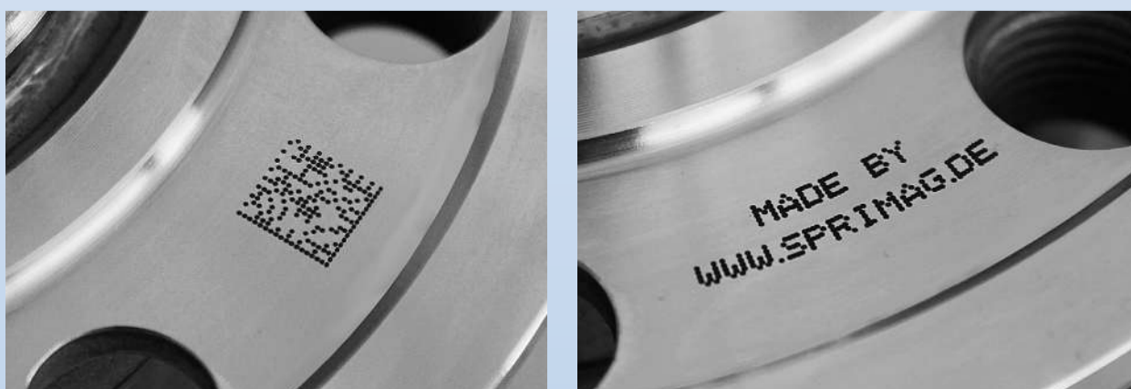
The Data Matrix Code is applied to the wheel bearings using inkjet
